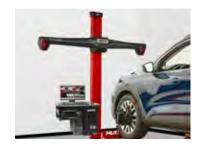
**Fixed-column configurations** fit most service bay applications.
